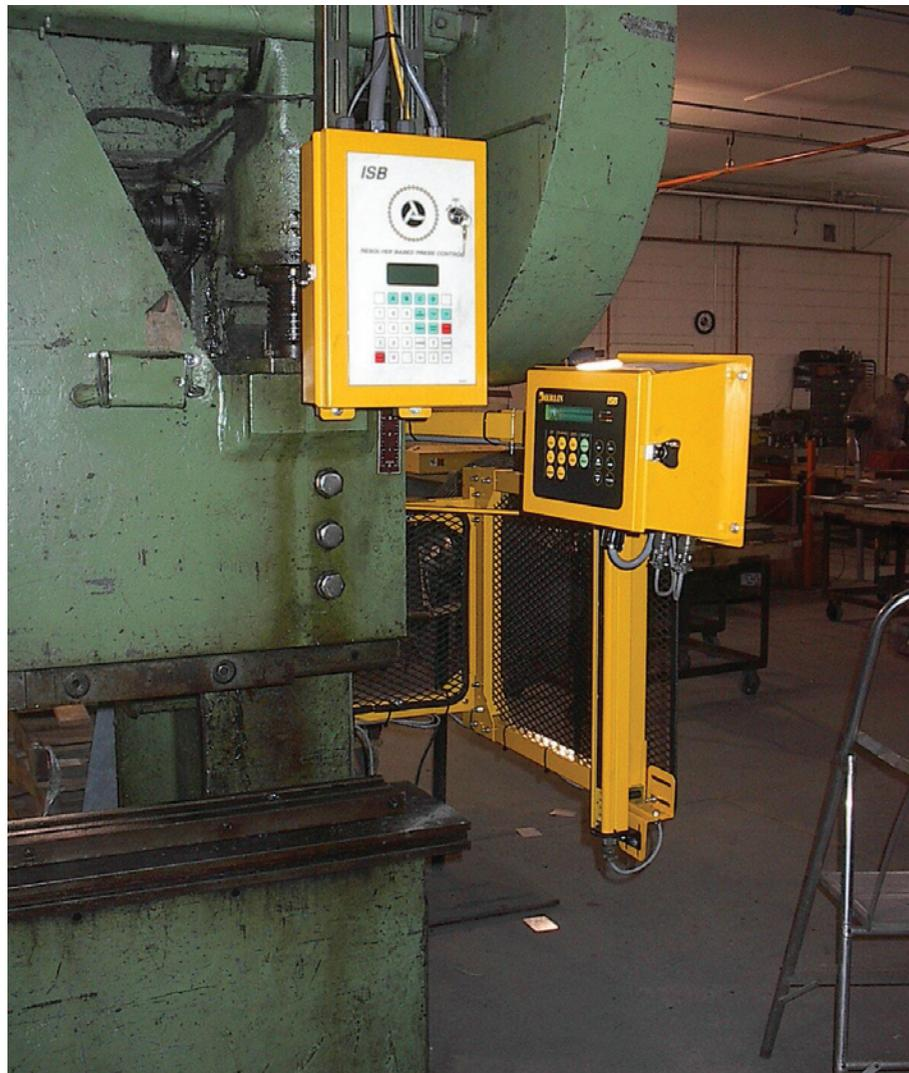
systems. Many of these earliest ISB Solid-State press controls are still in operation today and providing the highest level of control reliability.
