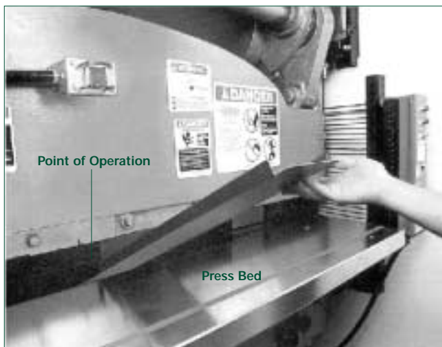
Figure 25 Power Press Brake Bending Metal
